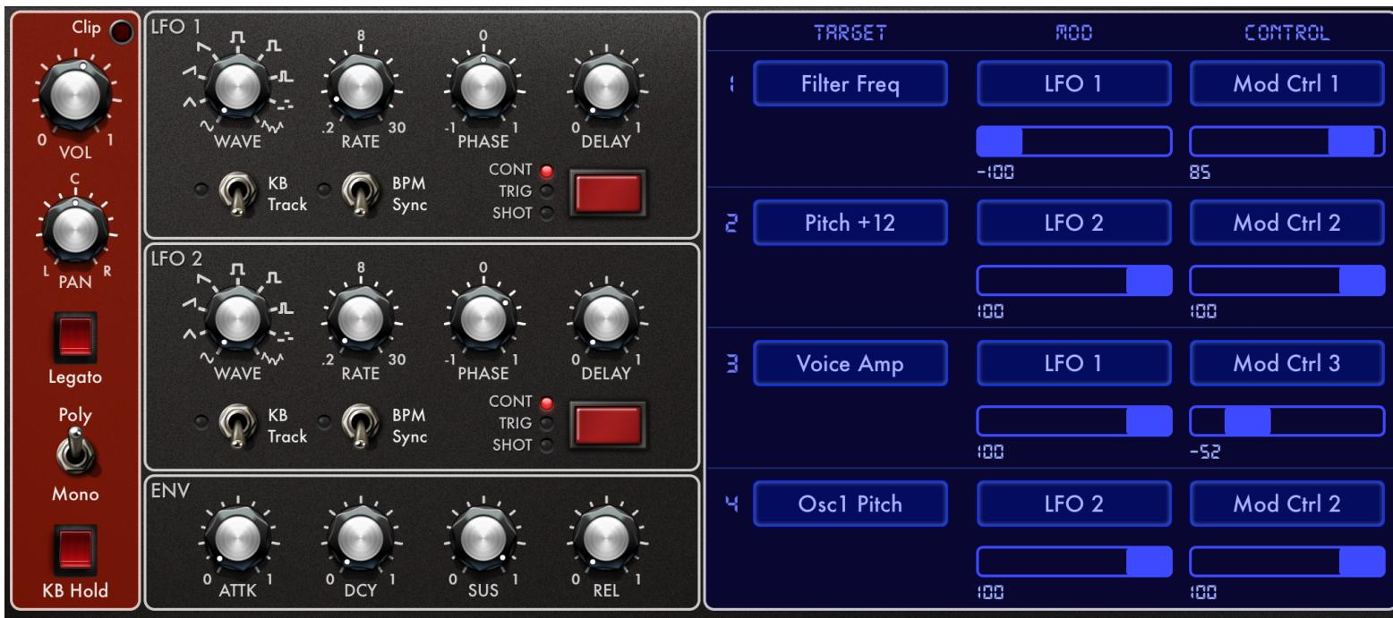
Kauldron features a versatile and easy-to-use modulation system to deliver interesting new textures and sounds. The two LFOs, the special modulation envelope, as well as a host of other control sources could be combined to manipulate synth parameters in real time, including via MIDI controllers.
